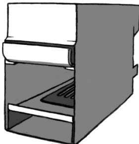
There is a grate cradle in the bottom of the heater. There is one grate in the cradle and on the top shelf there is a fire plate. The flames in the heater will be directed to the chimney behind this fire plate. It makes sense to remove these pieces for the installation so the heater is as light as possible. **The grate cradle and the fire plate must always be in their places when using the heater. (See picture on the left)**
