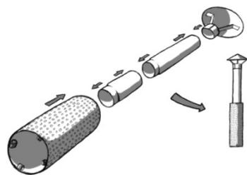
If you have purchased a chimney kit with the heater. It is supplied in a separate box and has four parts (see picture right) and it has to be assembled.
