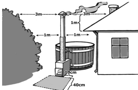
When positioned close to the roof or when taken through it, the top end of the insulated chimney must be at least one (1) meter above the surface of the roof. Ask your local fire officer for more information.
