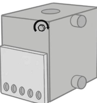
**NB! Before heating up check that the thread is waterproof. If water is leaking through the thread then fasten it more and check that o-ring is in place.**
